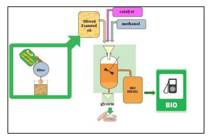
At first the oil is filtered to remove food residue, the filtered oil is put into the reactor with methanol and a base (usually NaOH sodium hydroxide). The reaction can be carried out at low temperature. From the reaction are obtained biodiesel and glycerin. The glycerin is not only a byproduct, but itself represents a useful product in the pharmaceutical and cosmetic industry.
